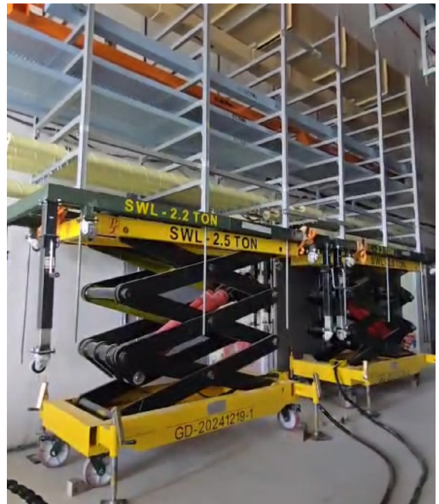
Synchronised lifter. (Photograph courtesy of Perfab Engineering Pte Ltd)
