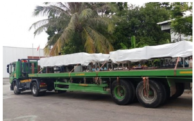
Figures 4 and 5: Completed modules properly wrapped in factory (top) and modules properly wrapped and secured for delivery to site (bottom). (Courtesy of Tech Onshore MEP Prefabricators)
